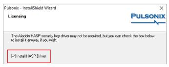
Once the installation is complete, if you connect the USB key, the Windows Plug & Play option will automatically detect the key and request the driver. Select the Aladdin HASP driver installed. The key will now be ready for use.
